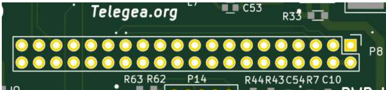
Illustration 13: Detailed View of the Extension socket for custom modules
