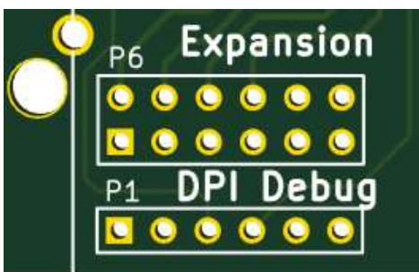
Illustration 9: Detailed View of the Generic Expansion and Debug Port Headers
