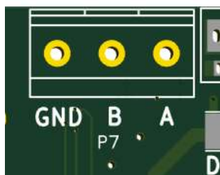
Illustration 3: Detailed View of Modbus Terminal
